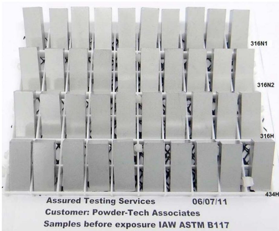
Figure 6: TRS bars in their racks prior to salt spray testing.
