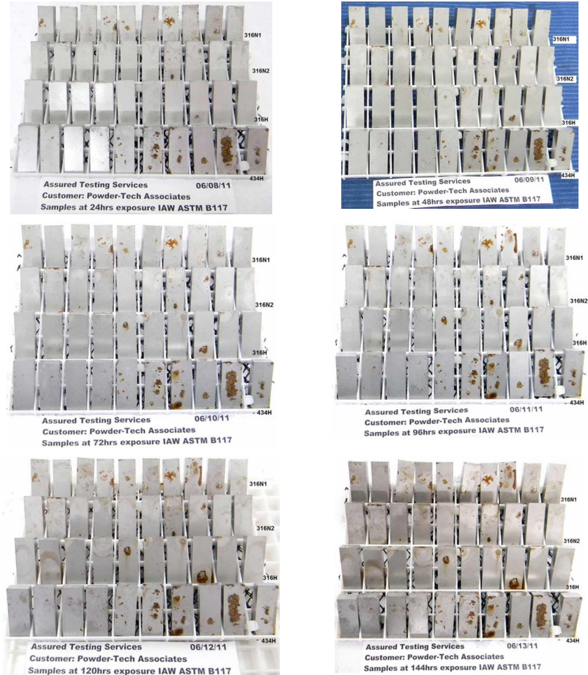
Figure 11: Photographs of the various test bars at different times of salt spray exposure.
